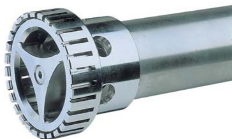
S 65 KG-HH-G65 M Volume: 2-40 litres Dispersion: 20-50 µm Emulsion: 5-15 µm
